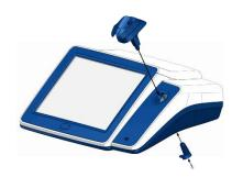
Place the mounting adapter in the insertion on the right-hand side of the device making sure the opening of the mounting adapter is pointing downwards.
